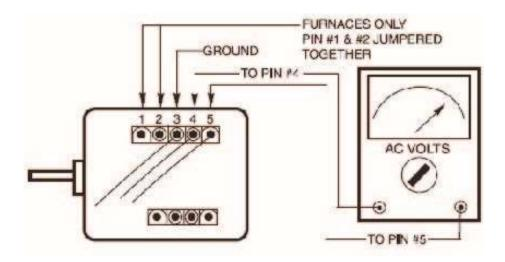
Yes - Remove the serial motor wiring harness at the IFC Apply 24 VAC to wires 3 & 4. See diagram #2 below Does motor run?
